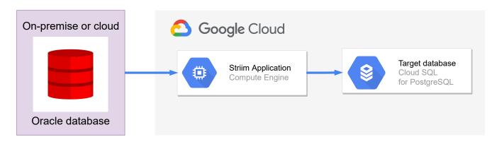
This architecture involves running the Striim application on a Compute Engine instance. It connects to an Oracle database that's hosted on-premises or in the cloud, and writes data to a Cloud SQL for PostgreSQL instance on Google Cloud.
