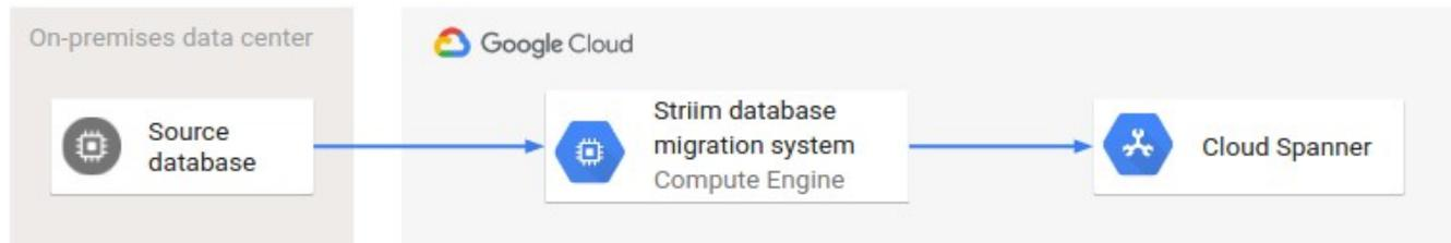
In this architecture, the source database system is migrated to the cloud-based database system, which in this case is Cloud Spanner. The database migration system, Striim, is connected to both systems and migrates the data from the source to the target database system.
