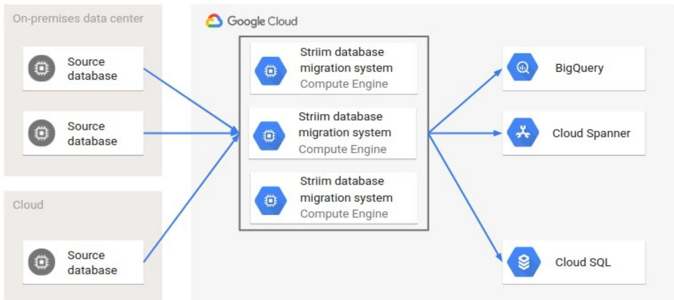
Three source databases are connected to Striim, and Striim migrates and replicates data to three target databases. The two source databases in the on-premises data center are replicated to BigQuery and Cloud Spanner, and the source database in the cloud is migrated to Cloud SQL.
