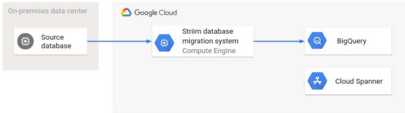
This scenario demonstrates that the deployment architecture is not necessarily static. Some use cases, like a one-time database migration, require that the migration system be connected to the systems or services until the migration is completed. Other use cases are more static, as in the case of database replication. This architecture shows how one architecture can serve several use cases.
