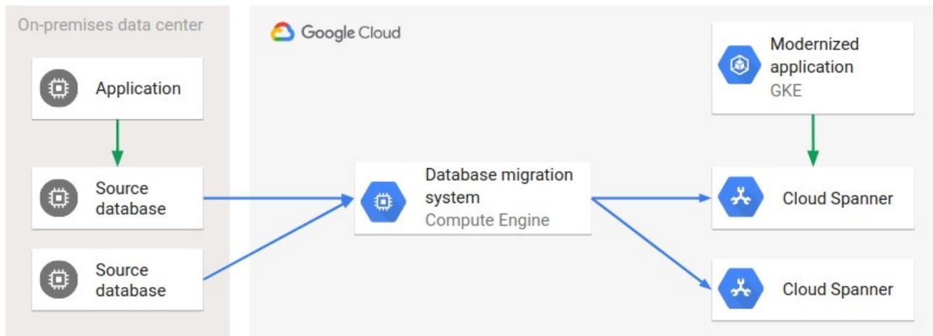
In this setup, two source databases are migrated to two target databases. One of the source databases is accessed by an application that accesses the corresponding target database in modernized form (implemented on Google Kubernetes Engine). The second source database also has clients (not shown in the diagram).
