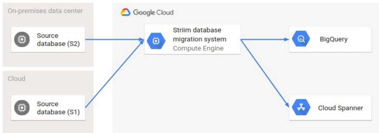
With the ability to transform and normalize data in streaming data pipelines, Striim can integrate a selected subset of the source transactional data to analytics platforms while the remaining data is continuously moved to one or more Google Cloud data targets.
